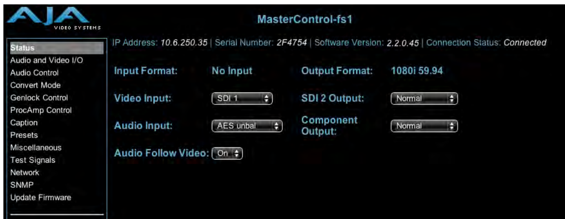
FS1 Web Interface, Main Status Screen
